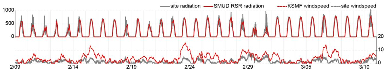
Figure 4. Comparison of solar radiation (left axis, W/m<sup>2</sup>) and wind speed (right axis, mph) between local and site weather stations.
