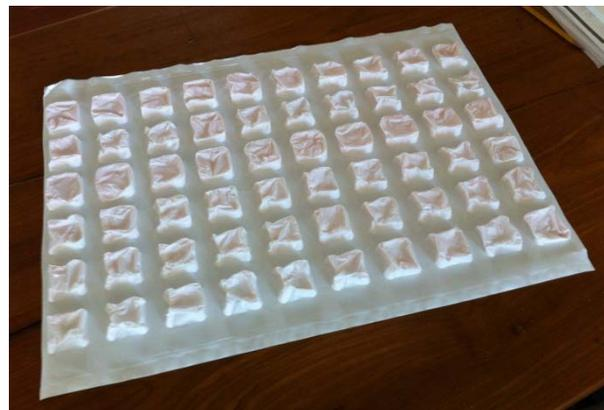
Figure 1 The PCM product tested in this study
